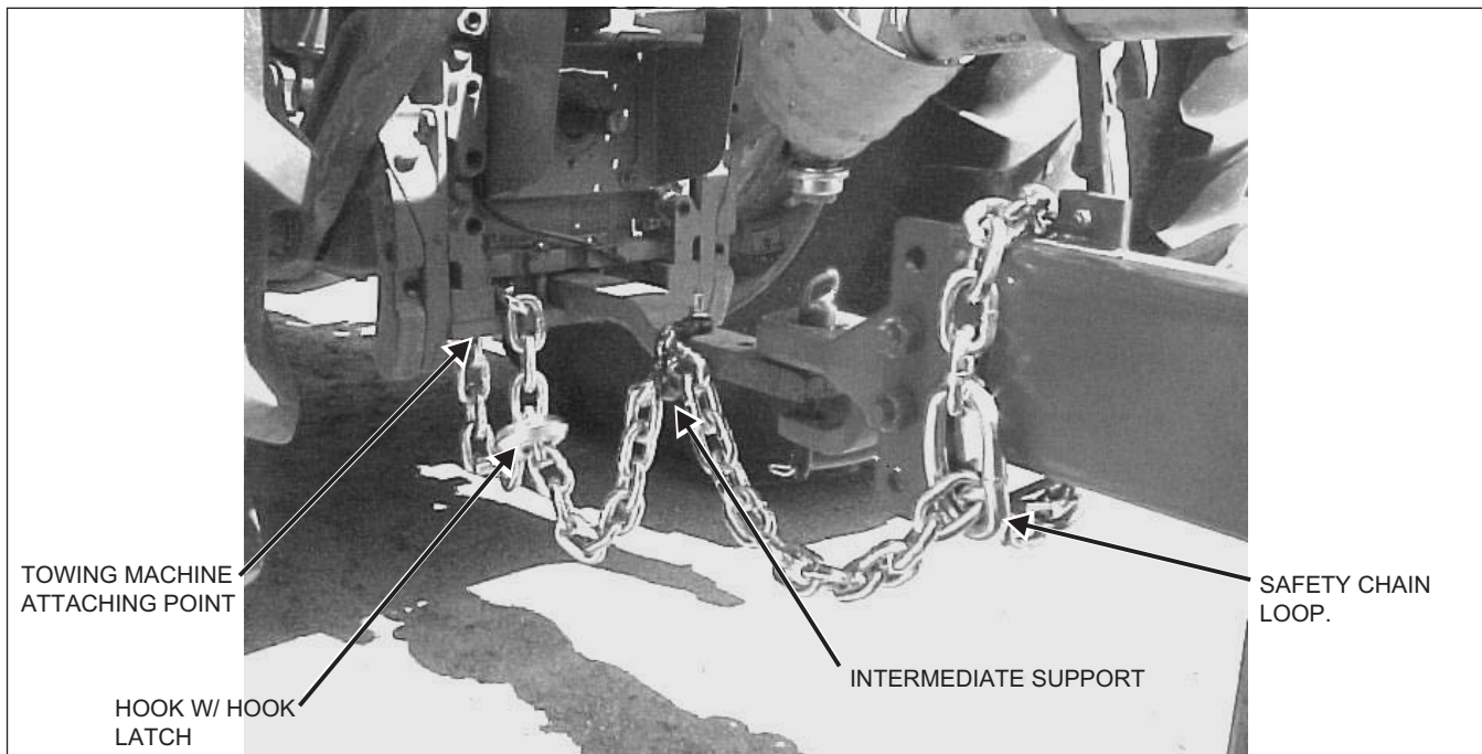
FIGURE 3. SAFETY CHAIN INSTALLATION
